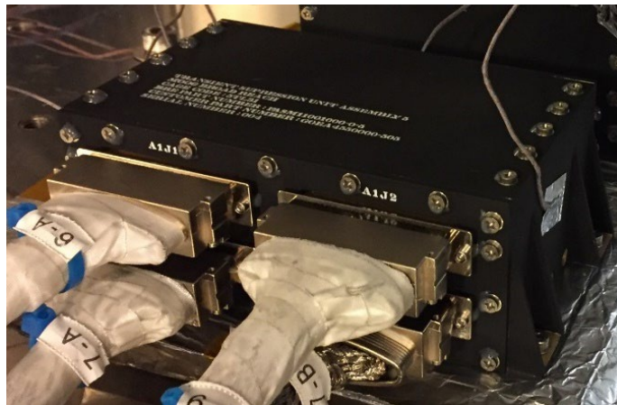
Figure 11-7. Transient Suppression Unit (TSU)
