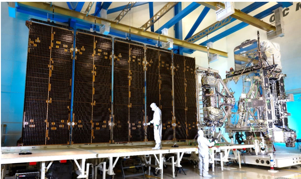
Figure 12-3. The Solar Array installed on GOES-16
